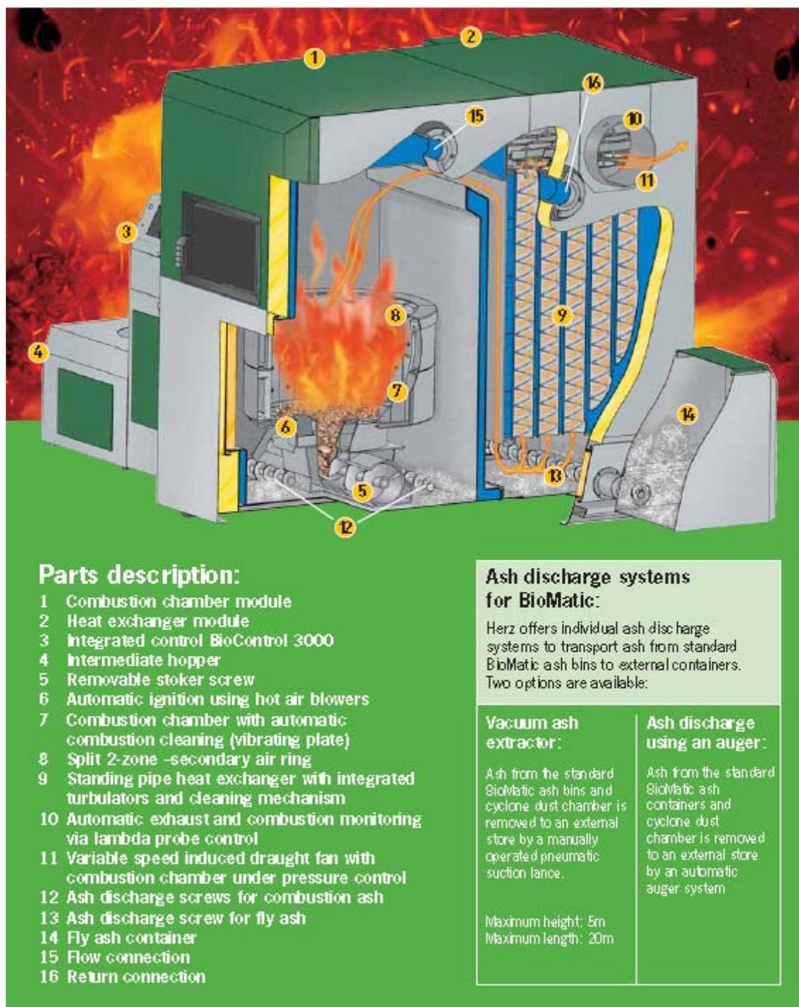
Figure 8: Herz BioMatic Boiler Diagram
