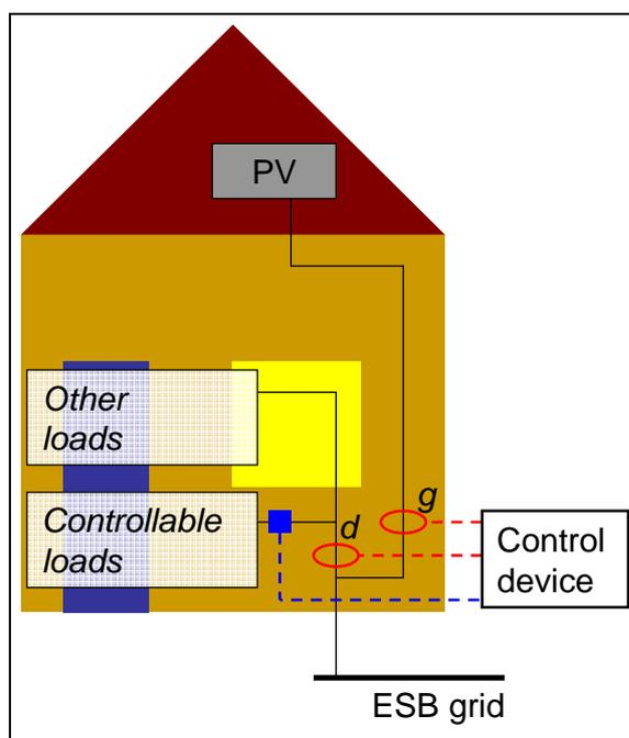
**Figure 3: Measurement and control points for individual properties**
