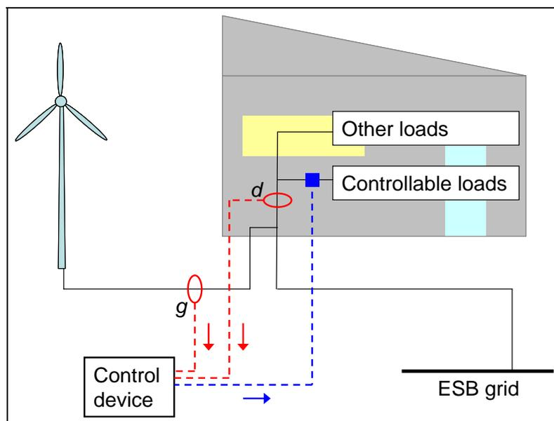
**Figure 2: Outline of measurement and control points for utility area.**
