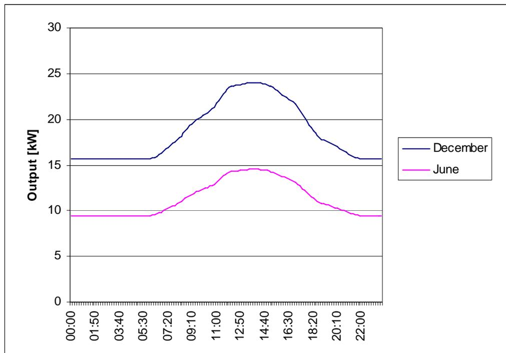
**Figure 6- Models for wind power output of a 50kW turbine operating at a 30% capacity factor**
