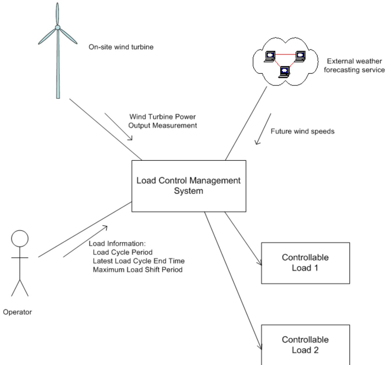
**Figure 9 – Load Control Management System**
