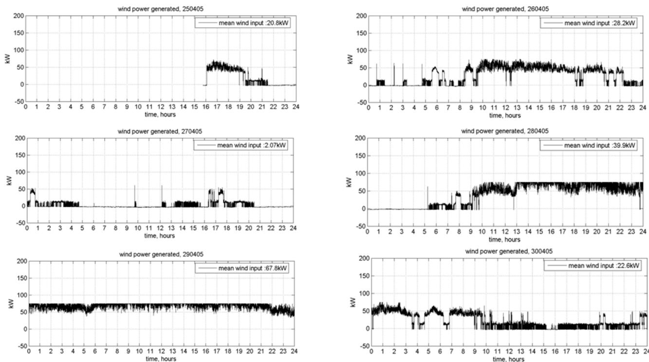
**Figure 5 – Variation of the mean power output of a 75kW wind turbine over six days**
