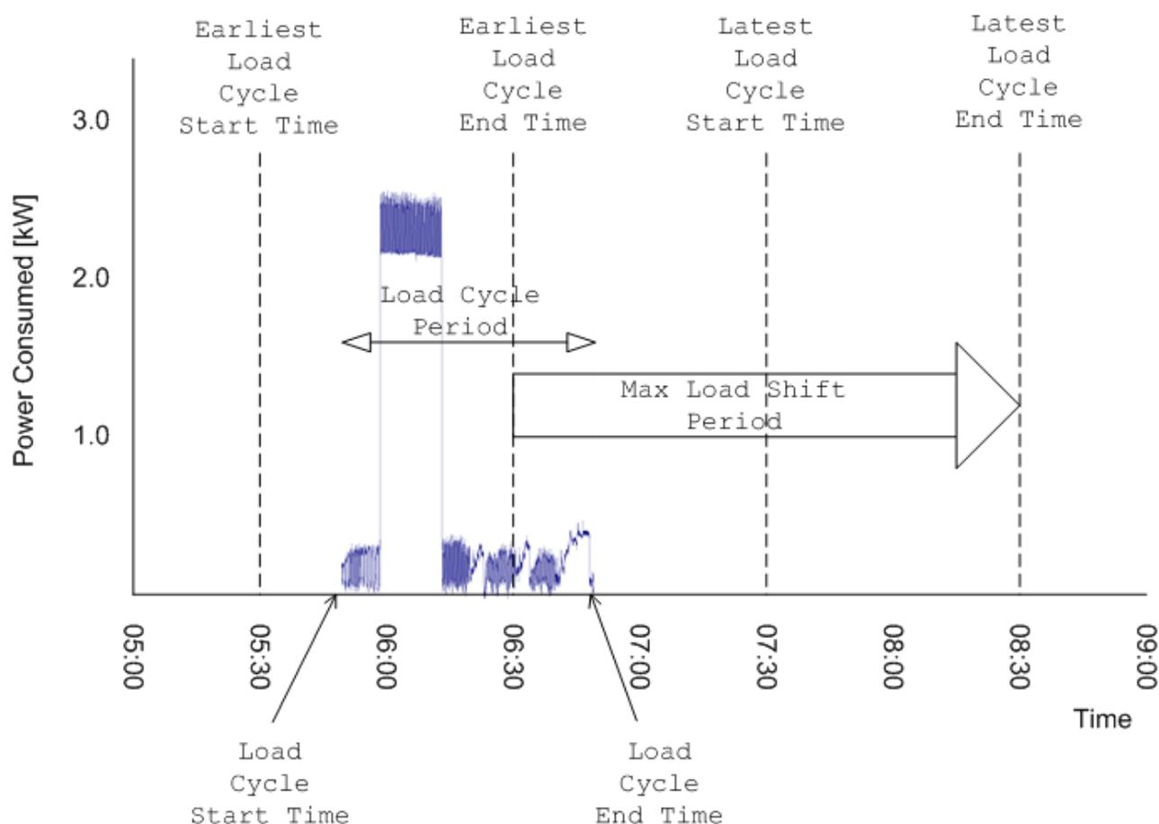
**Figure 7 – Washing machine demand profile used to explain load shifting terms and definitions**
